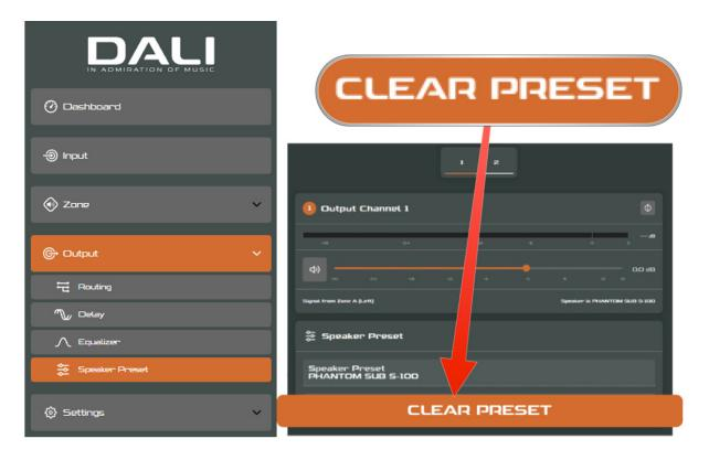
Now the AMP-2500 speaker preset section is 'unlocked', and you can use the built-in DSP tools to create your own speaker preset.
