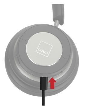
Connect the headphone to the computer using the USB cable.
