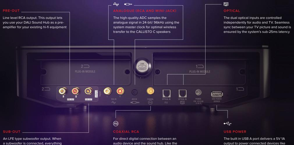
a subwoofer is connected, everything below 100Hz is sent via this output to a connected subwoofer For direct digital connection between an audio device and the sound hub. Like the optical input, it will accept signals from 16-bit/32kHz to 24-bit/192 kHz The built in USB A port delivers a 5V 1A output to power connected devices like Google Chromecast Audio, or charge a mobile device while playing
