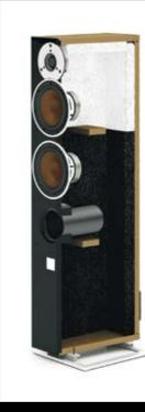
Cabinet | CNC machined MDF board, dressed in a top-of-the-class laminate forms the framework of the speaker. In addition, the floor-standing models feature strong internal bracing to reduce structural resonances.
