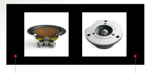
The 5¼" woofers in the ZENSOR AX series feature 4-layer voice coils for maximum control of the wood fibre cone. The low loss construction is ensured by a rigid metal basket and meticulously optimized cone. The result is bass authority, well-controlled reproduction of micro-detail and great transient capabilities.
