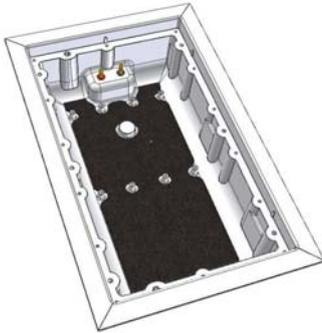
A rigid, die cast aluminium cabinet has been used for the IKON Phantom. This will ensure identical working conditions for the 6.5” bass/midrange driver no matter which wall cavity the speaker is mounted in. Inside the cabinet is used a bituminous material to make it inert to resonances. Ribs in the die cast aluminium and the coupling to the MDF baffle will also prevent build-up of resonances.
