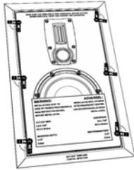
IKON Phantom comes with a cut-out template, which will make marking for the wall cut-out easy. Also, it can be taped to the wall to have a preview of the loudspeaker setup before the Phantoms are mounted.
