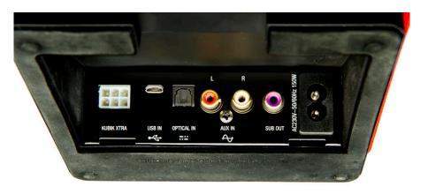
Most of the connectors on the KUBIK FREE are conveniently hidden away in the bottom part of the unit for easy placement on a wall or a flat surface.
