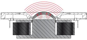
In the right light this fine fabric will reveal the soft felt damping on top of the pole piece. This damping material eliminates unwanted reflections that may occur from a traditional flat-surface pole piece, applied in simpler tweeter constructions. This is another example of the meticulous care for construction details that - altogether allow an unfiltered reproduction of all the details in the music.
